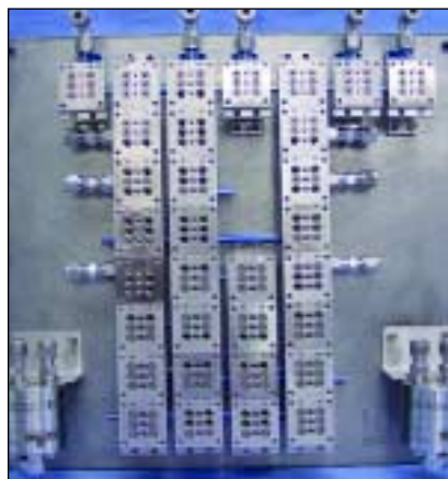
Figure 3. Hoke, Inc.'s \mu\text{MS}^3 modular sampling system. Unique to Hoke's components are silicon dioxide coatings, Silcosteel (300- \mu\text{m} thick) and Sulfinert (1,300- \mu\text{m} thick), that make the parts highly inert to moisture and sulfur, respectively.
