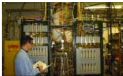
A 12-h/d pilot reactor in Westwood, MA, produces fullerenes using Nano-C's solvent-free combustion technology.
