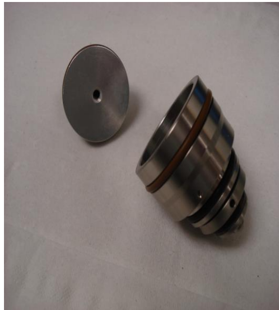
2.) Unscrew indicator from cartridge
