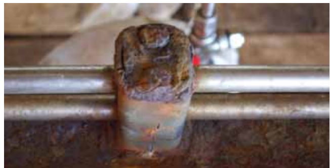
Crevice corrosion between the tube/tube trap interface.
