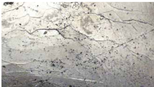
Stress Corrosion Cracking Stainless Steel in Seawater Environment
