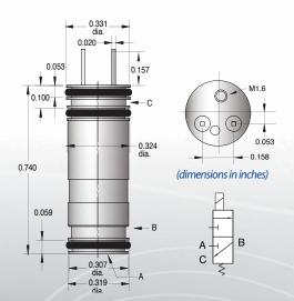
These new direct actuating valves offer an extremely fast response time for accurate dosing of minute volumes with the same long life you expect from the original Clippard EV line of electronic valves, now in a 8 mm cartridge package.
