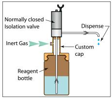
Maintaining a repeatable dispense of aggressive (and often very expensive) reagents into an analytical instrument can be problematic with conventional pumping equipment.
