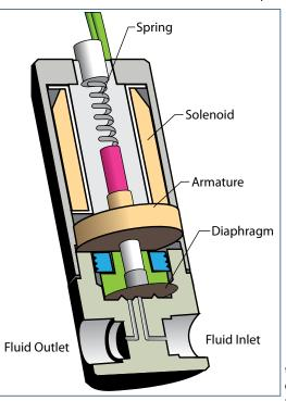
The valves use a flexible diaphragm to isolate the solenoid actuation mechanism from the fluid path. Isolation Valves are available in three different configurations: normally closed, normally open and 3-way. When the valve is energized, the solenoid retracts the armature that is attached to a flexible diaphragm. In a normally closed
