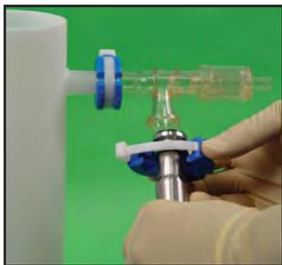
Position SaniSure Clamp around sanitary clamp fitting
