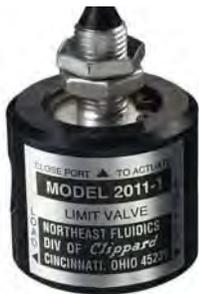
3-Way Bleed Pressure Piloted Limit Valve; blocking of the sensing port causes rapid valve opening
