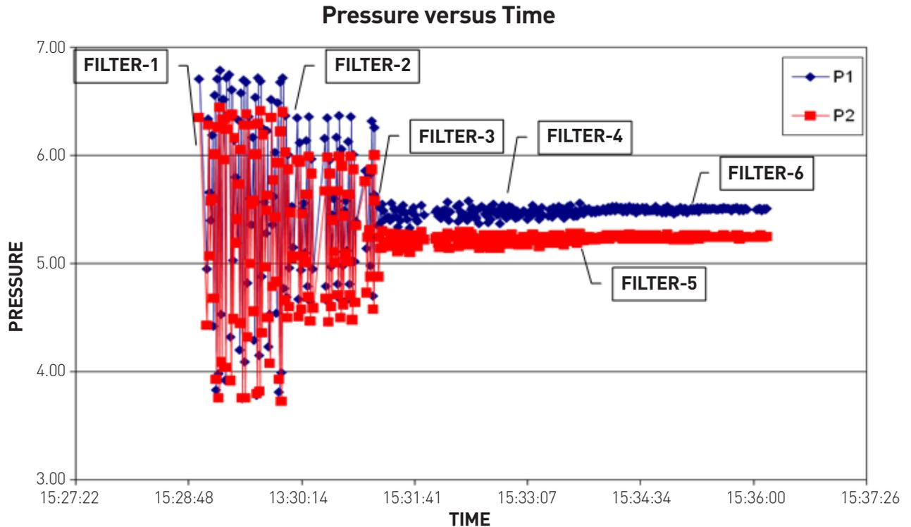
This graph shows the effects of the Filter setting on the SciPres® monitor and the incoming signal from the SciPres® sensors.
