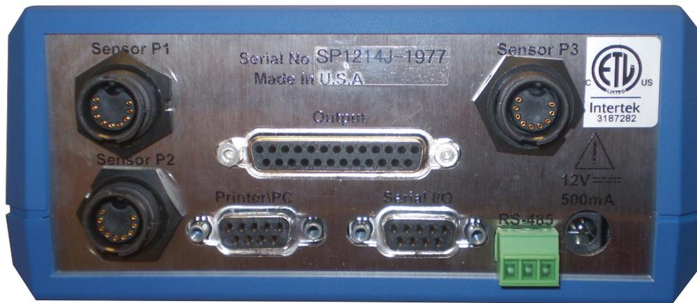
The SciPres® pressure sensor back panel provides interfacing ports for:
