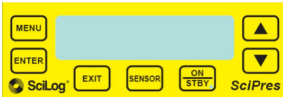
The front panel includes an alphanumeric display and a membrane keypad to select operational modes and alarm settings. The display is a two line, 20 character, liquid crystal display (LCD). The display is backlit to allow easy viewing over a wide range of lighting conditions.
