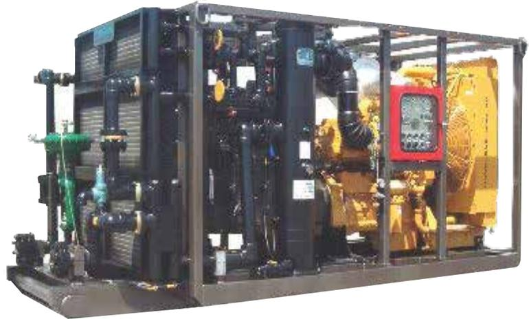
Diesel Powered Nitrogen Gas Booster with capacity from 300 - 1,000 SCFM (510 m<sup>3</sup>/hr) and outlet pressures from 350 - 5,000 PSIG (24 - 345 BARG)
