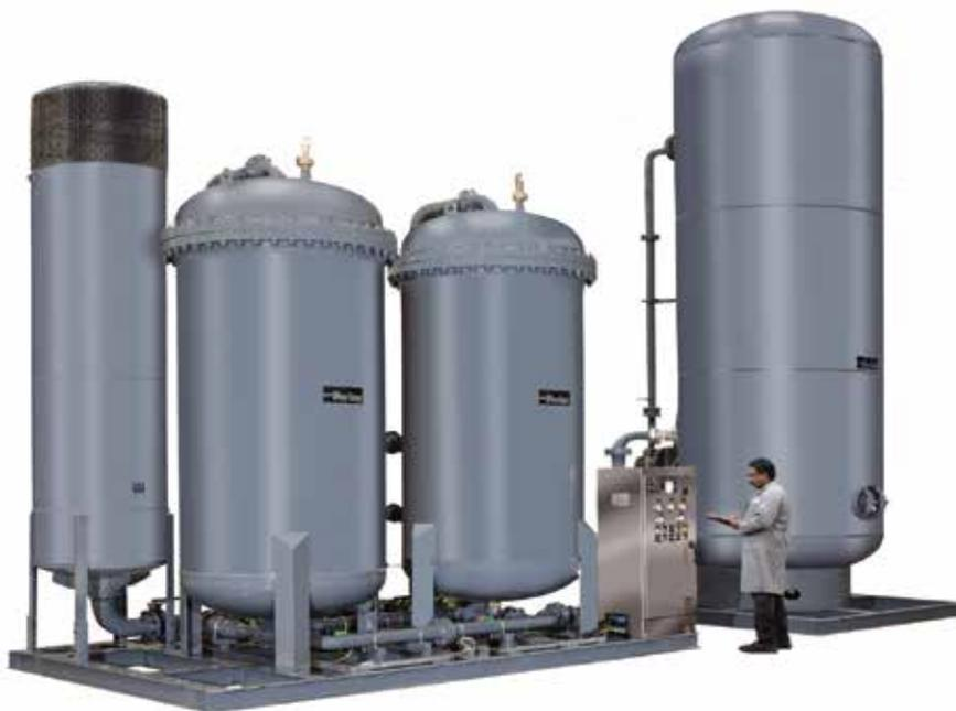
Large, Custom PSAs are available from nitrogen flow rates from 6,000 SCFH to 86,000 SCFH (170 m<sup>3</sup>/hr to 2435 m<sup>3</sup>/hr) from purities of 98% to 99.999%
